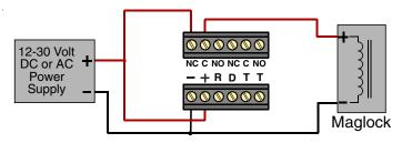
Relay contacts shown with Switch 3 ON (Failsafe Mode) and Power On
