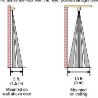
When the DS160/161 is mounted on the wall above the door, you can move the coverage pattern away from the wall by rotating the detector's lens.
