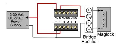
Relay contacts shown with Switch 3 ON (Failsafe Mode) and Power On.
