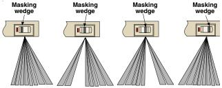
Insert a masking wedge by placing the bottom peg in first. Then press on the center of the wedge until it snaps into place.
